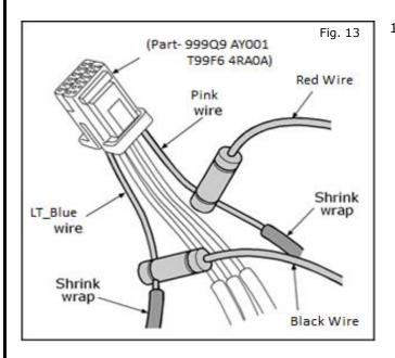
13. Using a posi-tap, connect the **Black** wire from the Kick Plate to the **LT\_BLUE** wire on the Accessory Connector Harness.
