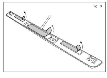
Carefully flip the driver Kick Plate over. Remove backing from three (3) adhesive strips located on the back of the Kick Plate.
