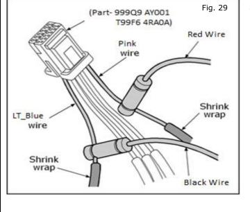
30. Using a posi-tap, connect the **Black** wire from the Kick Plate to the **LT\_BLUE** wire on the Accessory Connector Harness.
