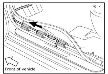
7. Feed the end of the wiring up through the existing harness clips towards the footwell.
