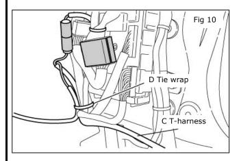
8) Attach the T-harness at the position shown in Fig10, using the tie wrap (D). (1piece)
