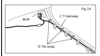
17) Route harness through existing vehicle harness protector and fix the harness at the position shown in Fig14, using the tie wrap (D). (3places)
