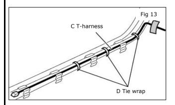
16) Route harness through existing vehicle harness protector and Tie Wrap (D) the harness at the position shown in Fig13. (3 places)
