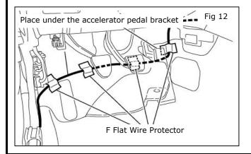
15) Flip the carpet of the driver's side and attach harness to floor using flat wire protector (F) shown in Fig12. (4places)
