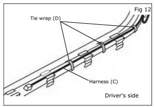
12) Route Harness (C) through existing vehicle harness protector and attach the Harness (C) to vehicle harness at position shown in Fig 12, using the Tie wrap (D)-(3 places)
