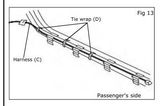
13) Route Harness (C) through existing vehicle harness protector and attach the Harness (C) to vehicle harness at the position shown in Fig13, using the Tie wrap (D) - (3 places)
