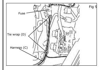
Attach the Harness (C) to vehicle harness at the position shown in Fig9, Secure by using the Tie wrap (D) - (2 places)
