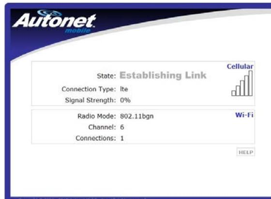
If you are unable to see the "Autonet-XXXX" in your wireless network list verify power is present to the WiFi module. If power is present and module still does not appear on the wireless network or the Establishing Link still appears on the display, access the following troubleshooting link:
