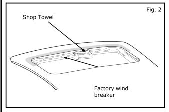
4) Push factory wind breaker down and insert shop towel to wedge it in place.
