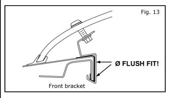
22) Push deflector forward to eliminate any gap between front brackets and flange.
