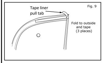
16) Fold tape liner pull tabs to outside of deflector and tape in place using masking tape.
