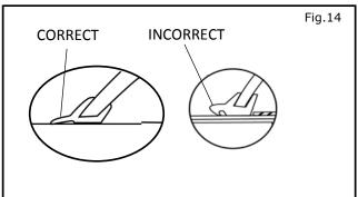
23) Check that rubber seal is not twisted or rolled under deflector. If necessary, slide a credit card under rubber seal to seat it correctly against roof.
