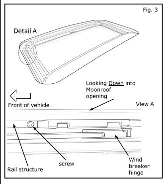
5) Locate small screw on rail structure near wind breaker hinge on drivers side.
