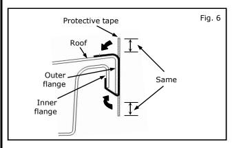
12) Peel protective tape from backing and locate evenly spaced as shown at final (4) locations.
