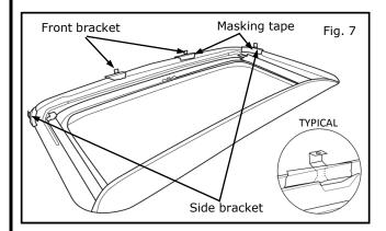
14) Center brackets on protective tape and secure in place with masking tape.
