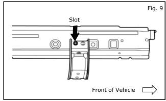
c) Locate one bracket to body sill in front location on driver side - use slot towards rear of vehicle. (Fig 9)
