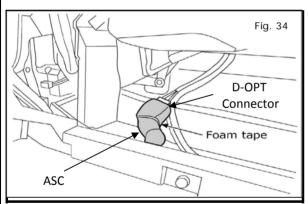
30) Plug the Accessory Service Connector (ASC) into D-OPT Connector plug on the Passenger side. Wrap the connectors in Foam tape to prevent rattle.
