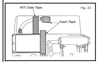
29) Wrap male connector in foam tape and secure to top of glove box with PET clear tape as shown. Add Foam tape over antennas.
