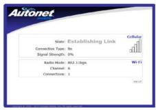
If you are unable to see the "Autonet-XXXX" in your wireless network list verify power is present to the WiFi module. If power is present and module still does not appear on the wireless network or the Establishing Link still appears on the display, access the following troubleshooting link:
