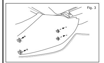
5) Install 1/4 turn fasteners at 4 drilled locations and rotate clockwise to engage.
