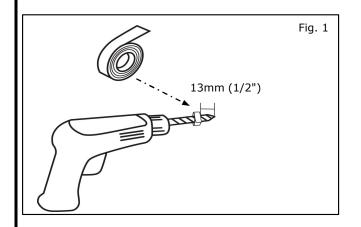
1) Wrap masking tape on 10.5mm (13/32") drill bit to limit drill depth to 13mm (1/2").
