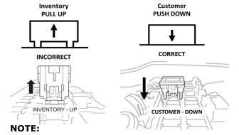
Typical vehicle condition shown above. Switch is easily identifiable by the permanent, push-pull fuse holder. Actual position on the fuse block may vary, vehicle to vehicle.
