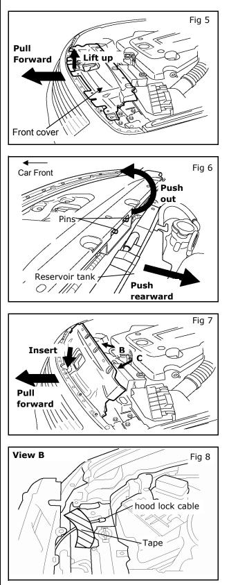
While pulling the top of the bumper forward, lift the front edge of the front cover up and sit it on the bumper. See Fig 5.
