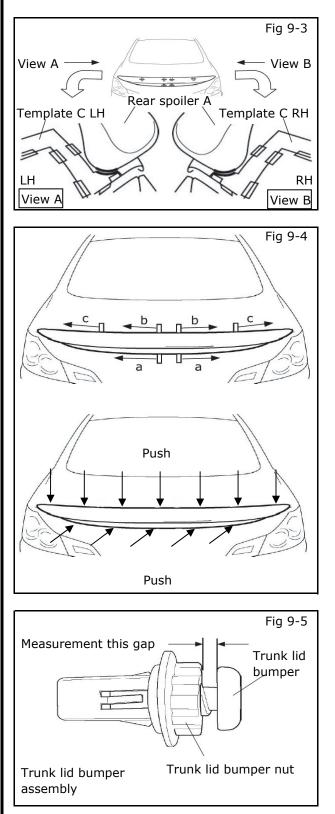
57) Position rear spoiler A equality clearance from aligning line of template C RH and LH.
