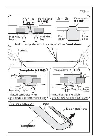
b) While referring to the illustration Fig 2, use masking tape and attach **template A LH** (E) to the front door's front bottom edge, **template B LH** (F) to the front door's back bottom edge and **template C LH** (G) to the rear door's back bottom edge.
