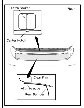
5) Align film into position with notch to latch striker and film edge against bumper edge.
