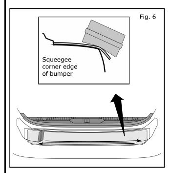
10) Firmly squeegee corner edge of bumper with three or four back and forth strokes in direction shown.
