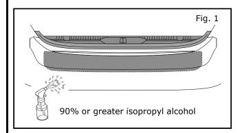
1) Using a clean lint free micro fiber cloth clean surface of rear bumper with 90% or greater isopropyl alcohol. Allow area to dry completely.
