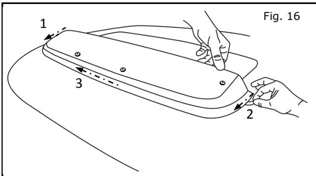
25) Fully tighten front bracket screws.
