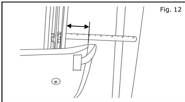
20) Remove masking tape from brackets and discard.
