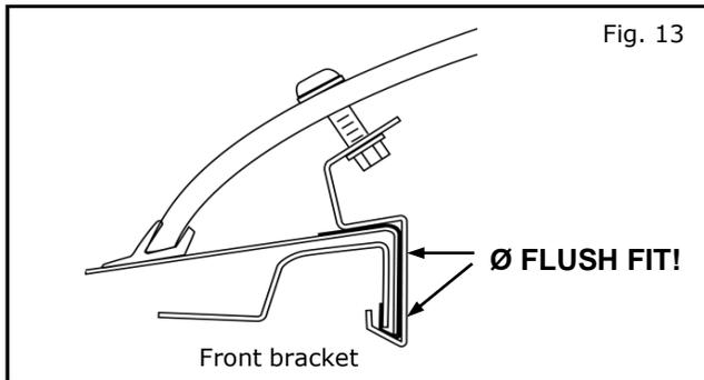
22) Push deflector forward to eliminate any gap between front brackets and flange.
