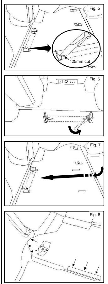
5) Using a **Utility Knife**, cut a 25mm (1") slit and pull back carpet to access bolts.
