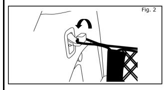
3) Attach net loops to upper hooks (driver side shown).
