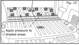
20) Apply pressure to shaded areas in figure 15 to secure hook and loop features.
