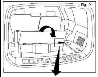
12) Place cargo bin lid in upright position, aligning lower hinge holes with vehicle holes.
