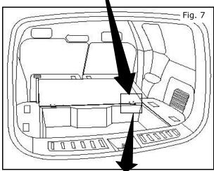
9) Align passenger side molded hinge assembly with holes on bottom of cargo bin lid.
