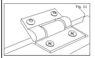
15) Ensure both molded hinge assemblies are attached with specified torque.
