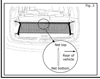
3) Attach cargo net hooks on the other side of the net to the D-rings on the driver's side.
