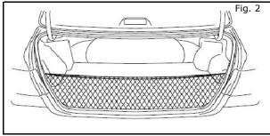
3) Attach the trunk net hooks on the other side of the net, to the D-rings on the driver side of the trunk.
