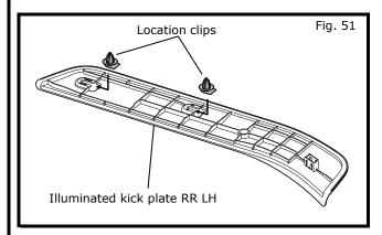
8) Slide Location clip into the clip seat of backside of Illuminated Kick Plate RR LH as shown in Fig.51.
