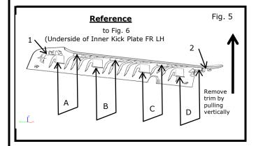
Important: Clips are located at locations labeled; 1, 2, and A thru D in Fig.5 and Fig.6. Note locations and orientations to avoid damage.
