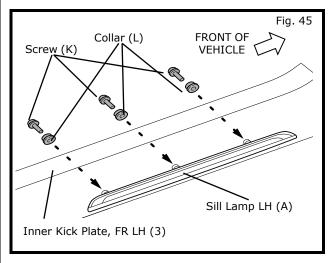
12) Secure Sill Lamp LH (A) with Collar (K) and Screw (L) to Inner Kick Plate, FR LH (3) as shown in Fig.45.
