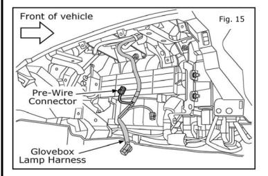
11) Inside the glovebox cavity, locate the Pre-Wire Connector on the glovebox lamp harness. Carefully cut the tape holding the connector and pull it out away from the harness.
