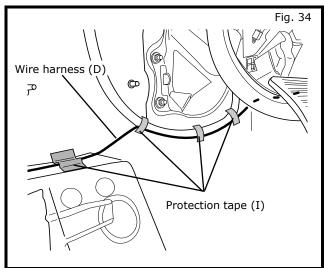
22) Route Wire harness (D) along vehicle parking brake cable as shown in Fig.34.
