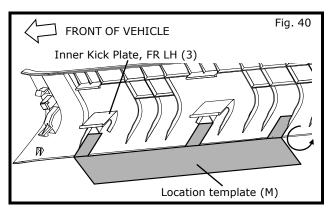
3) Align Location template (M) to Inner Kick Plate, FR LH (3) and apply masking tape to hold Location template (M) as shown in Fig.40.
