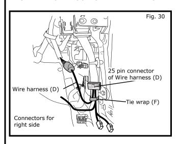
15) Route Wire harness (D) and secure to vehicle's harness by Tie wrap (F) as shown in Fig.30. (1 place)
