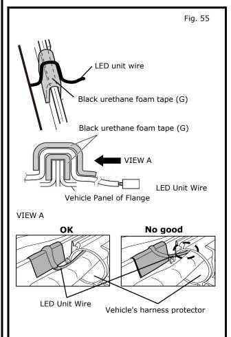
Place Black urethane foam tape (G) over flange, Then place the LED unit wire on top of the Black urethane foam tape (G) as shown in Fig.55. Apply second Black urethane foam tape (G) on top of the LED unit wire as shown in Fig.55.
