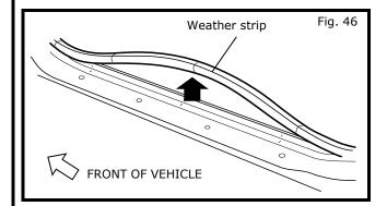
1) Remove the vehicle weather strip as shown in Fig.46.
