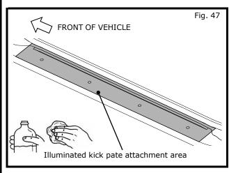
2) Clean the Illuminated kick plate attachment area as shown in Fig.47 with 50/50 alcohol & water, let dry for 30 seconds.
