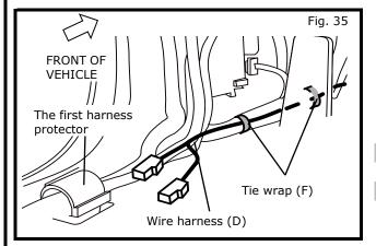
23) Route Wire harness (D) along vehicle's harness in front of the first harness protector of vehicle as shown in Fig.35.
