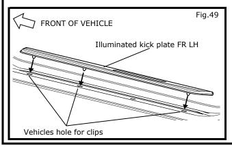
5) Align Location clips on part to first, second and fourth hole on vehicle from front side as shown in Fig.49.
