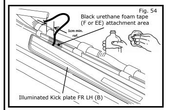
1) Clean both sides of the attachment area for the Black urethane foam tape (F or EE) with 50/50 alcohol & water, let dry for 30 seconds as shown in Fig.54.
