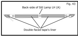
9) Do not remove double-faced tape liner located on back side of Sill Lamp LH (A) as shown in Fig.43.
