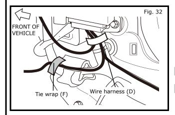
19) Route Wire harness (D) and secure Wire harness (D) to vehicle's harness by Tie wrap (F) as shown Fig.32. (1 place)
