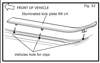
Tuck IKP under the door seal and align Location clips on part to first, second and third hole on vehicle from front side as shown in Fig.52.
