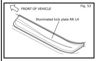
10) Insert Location clips to vehicles hole's and carefully push to lock clips
