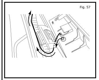
4) Route Sill Lamp wire through opening in carpet, then route Sill Lamp wire behind harness protector before making connection as shown in Fig.57.
