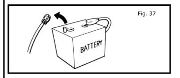
k) Disconnect battery as shown in Fig.37.
