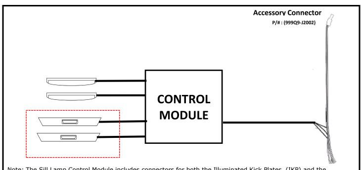
Note: The Sill Lamp Control Module includes connectors for both the Illuminated Kick Plates (IKP) and the Inner Sill Lamps. If IKP is already installed, it will use a separate jumper harness to the accessory connector. Do not remove the IKP jumper if was already installed since this will damage the accessory connector.
