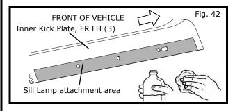
8) Clean the Sill Lamp attachment area as shown in Fig.42. with 50/50 alcohol & water, let dry for 30 seconds.
