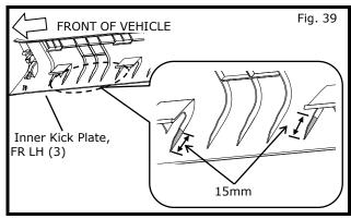
2) Cut the ribs of back side of Inner Kick Plate, FR LH (3) as shown in Fig.39.
