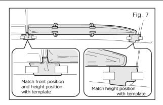
d) Align the RR side guard molding - LH (B) to the templates as shown Fig 7.
