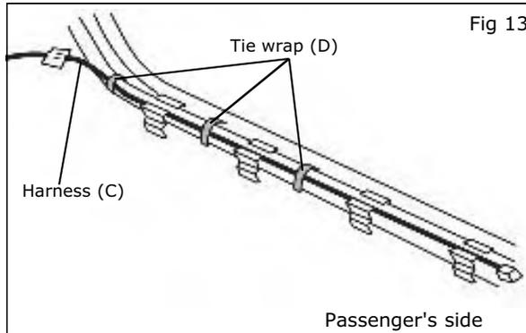
13) Route Harness (C) through existing vehicle harness protector and attach the Harness (C) to vehicle harness at the position shown in Fig13, using the Tie wrap (D) - (3 places)
