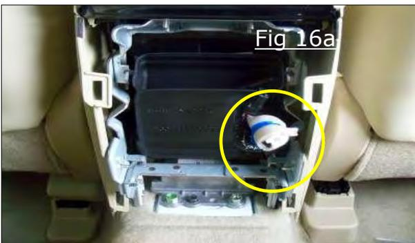
23) Locate factory connector for Aux In harness. Figure 16a
