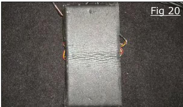
32) Place (1) 4"x8" piece of foam tape on top side of control box and double sided tape on bottom of control box. Figure 20
