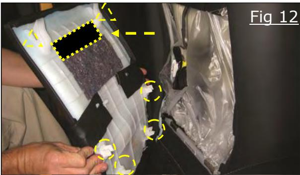
18) By hand pull the bottom side of the driver's seat back board releasing (4) clips. Slide panel down to clear catch tabs and remove. With seat back in hand, attach (1) 2"x6" piece of seat back foam tape as shown. (prior to re-installation) Figure 12
