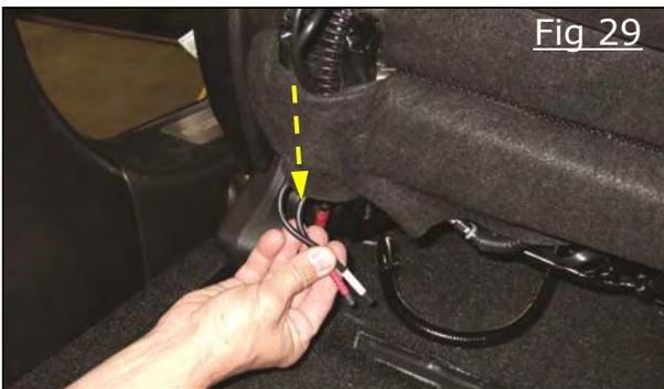
42) Continue to route cables through the carpet loop of seat following the factory wiring. Pull all slack through. Figure 29
