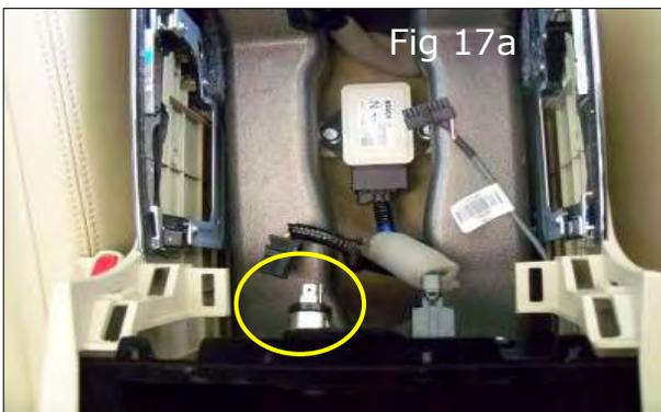
27) Locate and disconnect the power socket connector. Figure 17a
