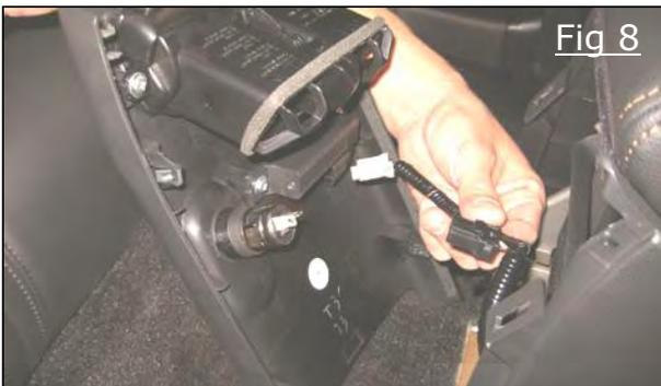
14) Disconnect electrical connectors from rear panel. Figure 8
