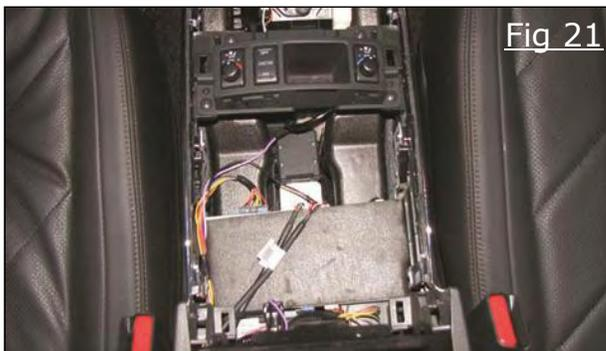
33) With all cables protruding rear of vehicle secure control box to the HVAC ducts in center console using double sided tape. Figure 21
