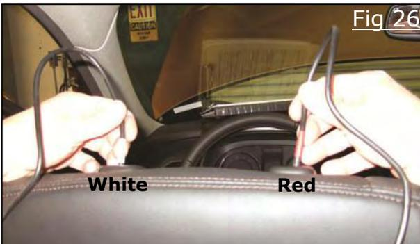
39) Insert cables # 1A and # 2A (white/ red) into the appropriate post holes of the driver's seat. Figure 26
