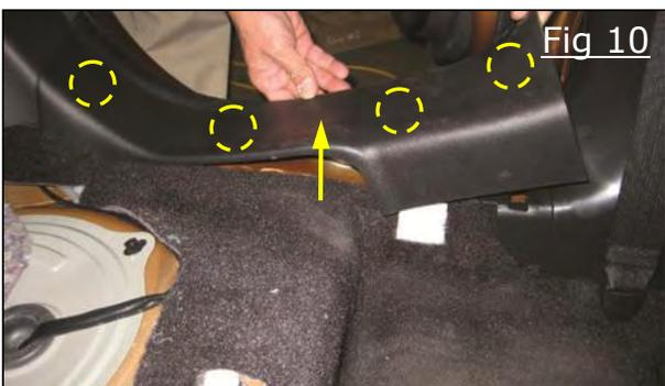
16) Pull up on the driver's side rear kicking plate to remove. Figure 10
