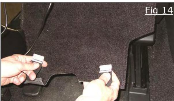
20) Reach under seat to release (2) plastic catches of the seat flap. Figure 14
