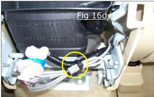
26) Wrap excess audio cable bundle to factory harness, foam is not required. Figure 16d
