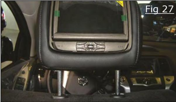
40) Continue to feed cables into seat until DVD headrest is in its highest locking position. Figure 27
