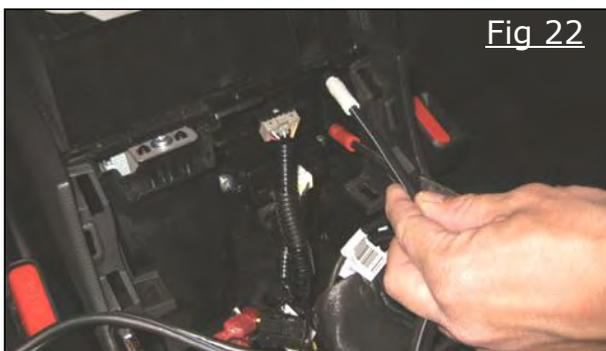
34) Feed cables # 3A down the driver's interior of the center console and exiting at rear of console. Figure 22
