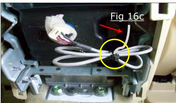
25) Route audio cable along with factory harness forward to center console finisher. Then wrap excess cable with cable tie, foam is not required. Figure 16c
