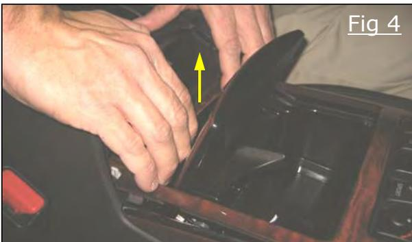
11) Open cup holder lid. From inside the cup holder cavity, pull up by hand to release rear clips of console finisher assembly. Continue forward to release remaining clips then clear shift lever from boot. Figure 4 & 5
