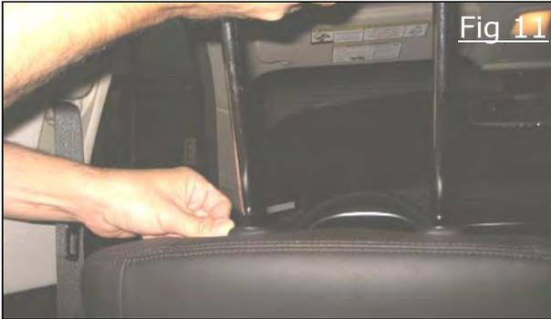
17) Remove driver's side headrest by depressing release button on left hand post coupler and pulling headrest up. Figure 11
