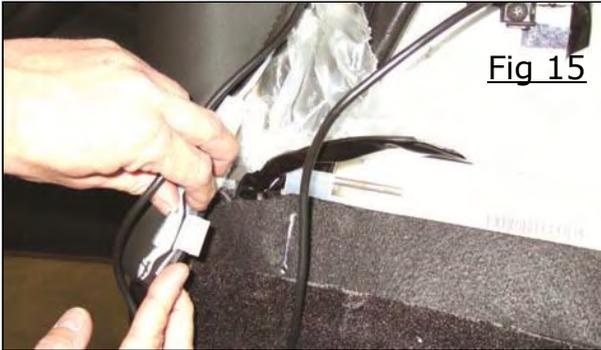
21) To allow for wire routing, release both clips holding the bottom left corner of the seat bolster. Figure 15
