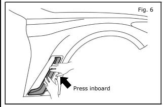
12) Uniformly press fender vent to fender and hold for thirty (30) seconds.
