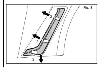
10) Remove remaining tape liners from outboard edges in order shown. Remove liners by pulling tabs away from fender vent.
